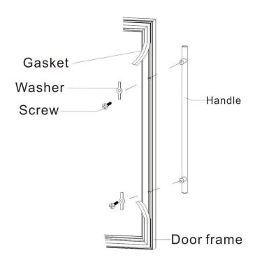
• Insert the washer and screws into the two slots on the inside of the door. Please note the washer must be inside the slot and screws pass trough the door frame.
